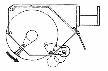
Where the size of the material to be cut makes it necessary for the front hood and carrier plates to be removed to allo with rotor to cut, the rotor must always be set to cut with downwards rotation – this results in a poorer finish to the work and demands higher power requirement.
