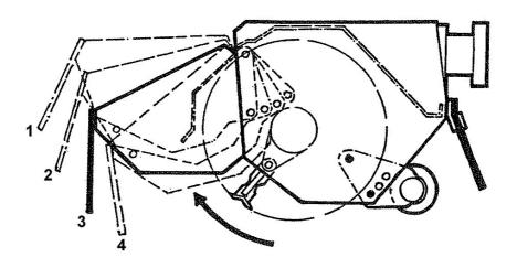
For mowing work the rotor must always cut with an upwards rotation and the roller set to a working height that is below the level of the skids *(or rotor if skids are not fitted)* - i.e. in position 2, 3, 4 or 5 as shown on the previous page.
