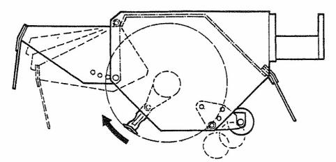
For normal trimming work on hedges the roto r should be set to cut with an upwards rotation – this produces a better finish to the work and demands lower power requirement. Front hood and rear flap must always be in position.
