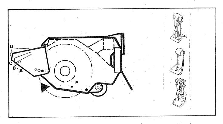
For the best finish the rotor should cut with an upwards rotation.
