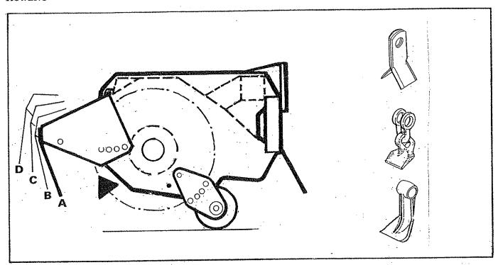
When mowing the rotor must always cut with an upwards rotation.
