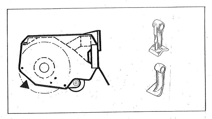
Where the size of the material to be cut makes it necessary for the front hood to be removed to allow the rotor to cut, the rotor must always cut with a downwards rotation.
