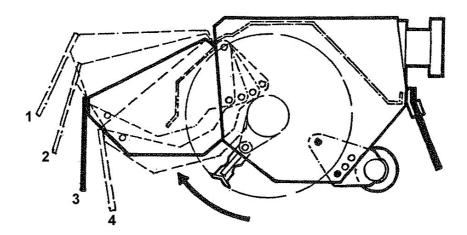
For mowing work the rotor must always cut with an upwards rotation and the roller set to a working height that is below the level of the skids *(or rotor if skids are not fitted)* — i.e. in position 2, 3, 4 or 5 as shown on the previous page.
