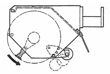
Where the size of the material to be cut makes it necessary for the front hood and carrier plates to be removed to allow the rotor to cut, the rotor must always be set to cut with downwards rotation – this results in a poorer finish to the work and demands higher power requirement.
