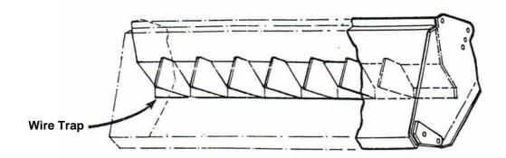
The flailhead is equipped with a 'wire cuttin g' edge welded into the undersid e – this pla te should not be interfered with in any way. If wire becomes caught in the rotor the machine must be switched off immediately and the wire removed.
