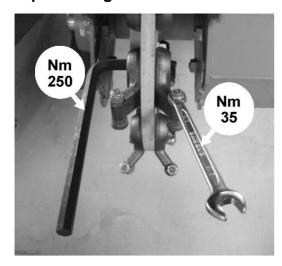
The correct torque settings for wear parts are shown opposite.
