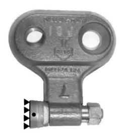
Best results are achieved when the outer edges of the grinding teeth are sharp. The grinding teeth can be rotated to position a fresh sharp edge outermost (3 x 120°).
