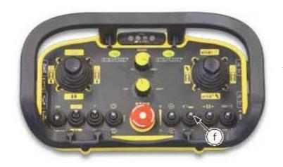
Angling of the machine to the left or the right is controlled by the use of switch 'f' indicated opposite.
