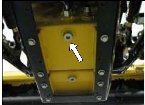
Hydraulic oil tank drain plug
