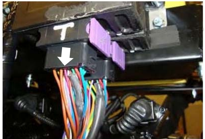
Disconnect the wiring loom plug from the Brake Control Module to allow machine operation with Manual Control
